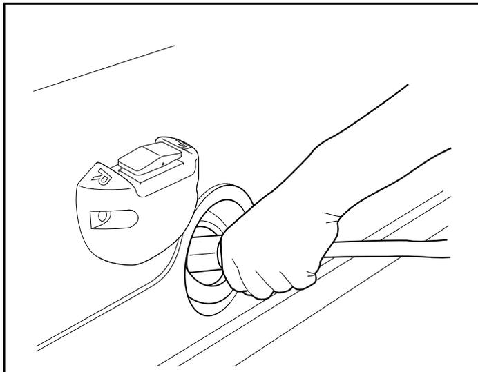
66 **Figure 28 Correct Insertion of Charger DC Plug**
