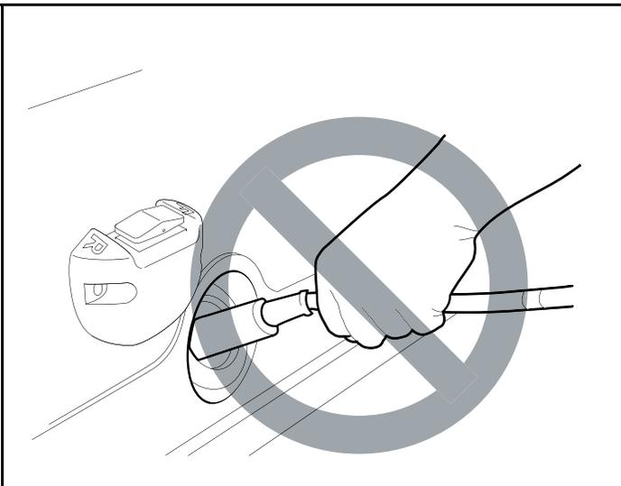
67 **Figure 29 Incorrect Removal of Charger DC Plug**
