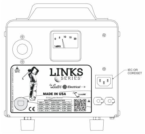
Figure 9.2-1: Links Series Model 27700 User Interface
