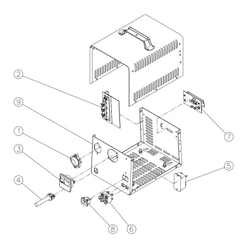
Figure 12-1: Links Series Model 27700 Service ISO View
